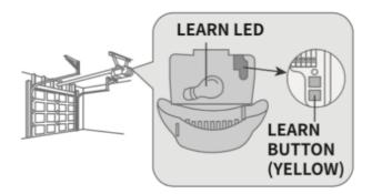
Within 30 seconds, press and HOLD below remote control button(bottom right one) until the garage door opener light flashes or clicks are heard to indicate successful programming.
